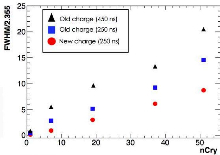
Noise width in the new charge increase linearly with the number of crystals added
