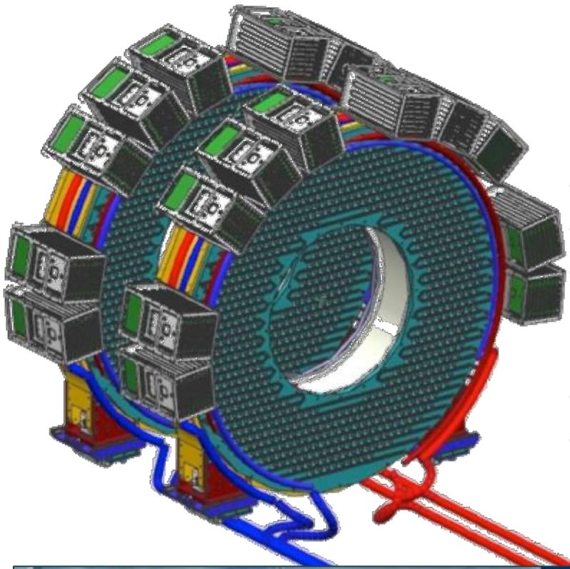
Two annular disks with 674 undoped CsI (34 x 34 x 200) mm<sup>3</sup> square crystals each
