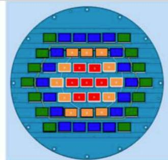
Cosmic trigger used to provide the equalization of all channels
