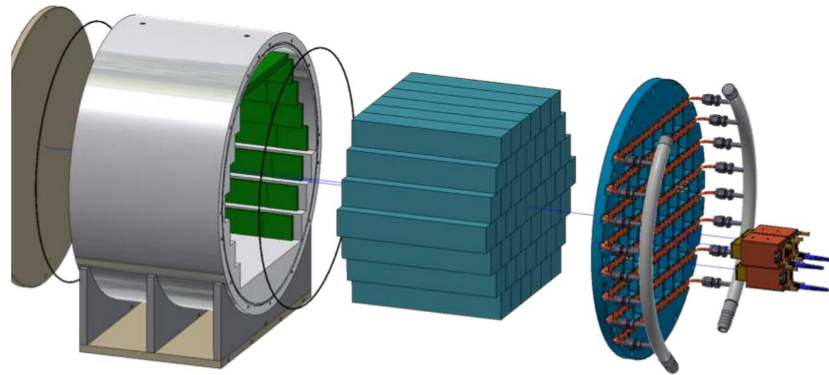
**Large size prototype: 51 crystals coupled to 102 sensors**
