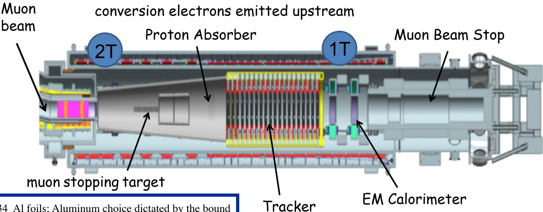
34 Al foils; Aluminum choice dictated by the bound muon lifetime (**864 ns**) that nicely matches the the Mu2e pulsed beam structure for prompts' separation
