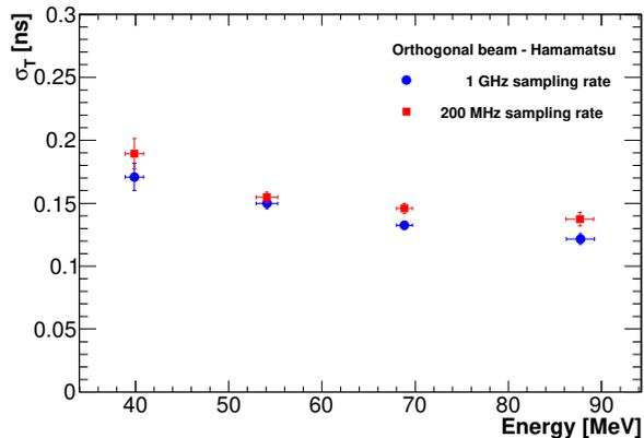
Figure 3: Time resolution as a function of the deposited energy in the highest energetic crystal, considering both the 1 GHz (blue points) and 200 MHz (red square) sampling rates.
