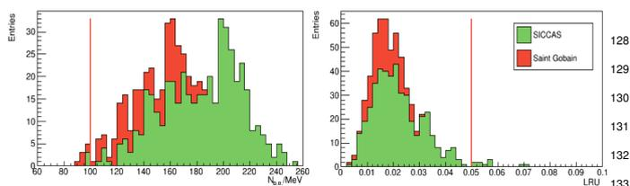
Figure 4: LY and LRU of about half of the crystal production.
