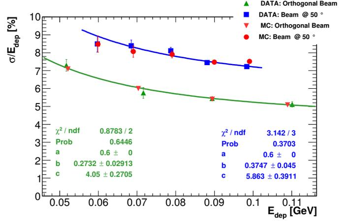
Figure 2: Energy resolution as a function of the deposited energy in Module-0. Green (blue) points are the results for the beam impinging at 0 (50) degrees. Red points are the results from MC simulation.
