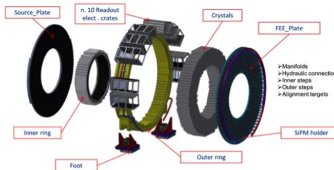
Figure 7: Exploded view of a calorimeter disk mechanic.
