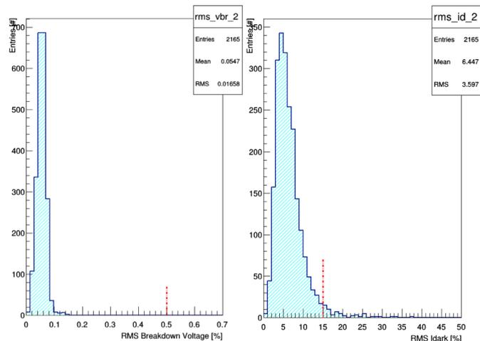
Figure 5: RMS distributions of the  $V_{br}$  and  $I_d$  measurements over the six cells of the Mu2e-SiPMs arrays.
