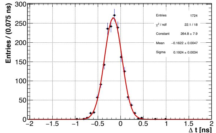
► Cosmic equalization provide **energy res at the level of 5 %**
