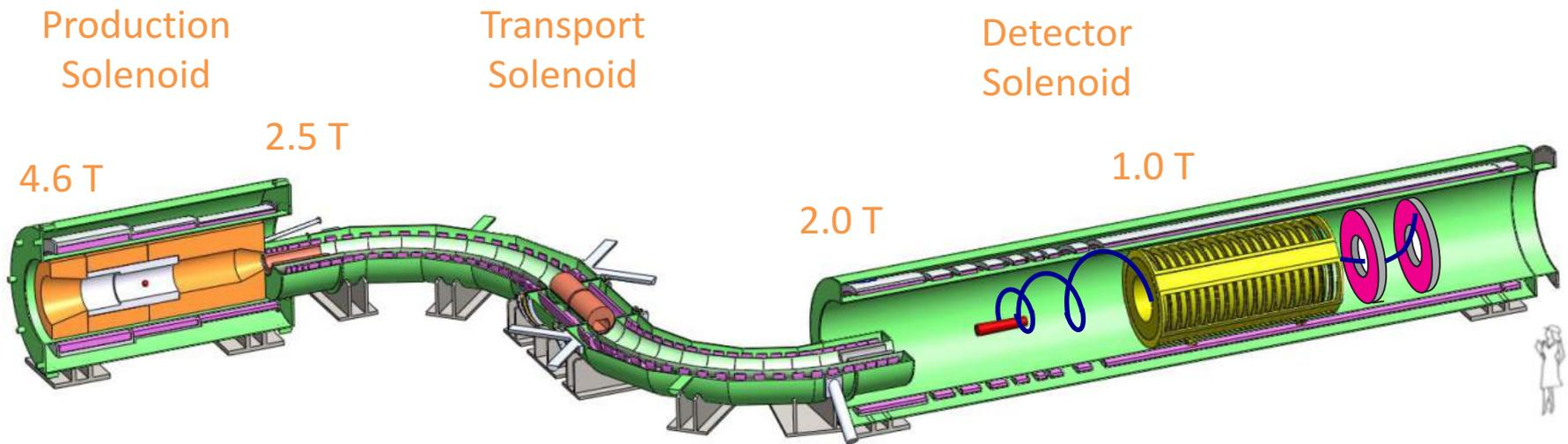
Graded fields important to suppress backgrounds, to increase muon yield, and to improve geometric acceptance for signal electrons
