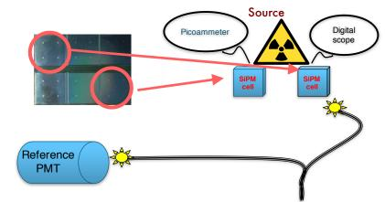
➡ 1 cell used to measure Idark and the other to monitor the Gain ➡ One PMT was used as reference for the Gain measurement
