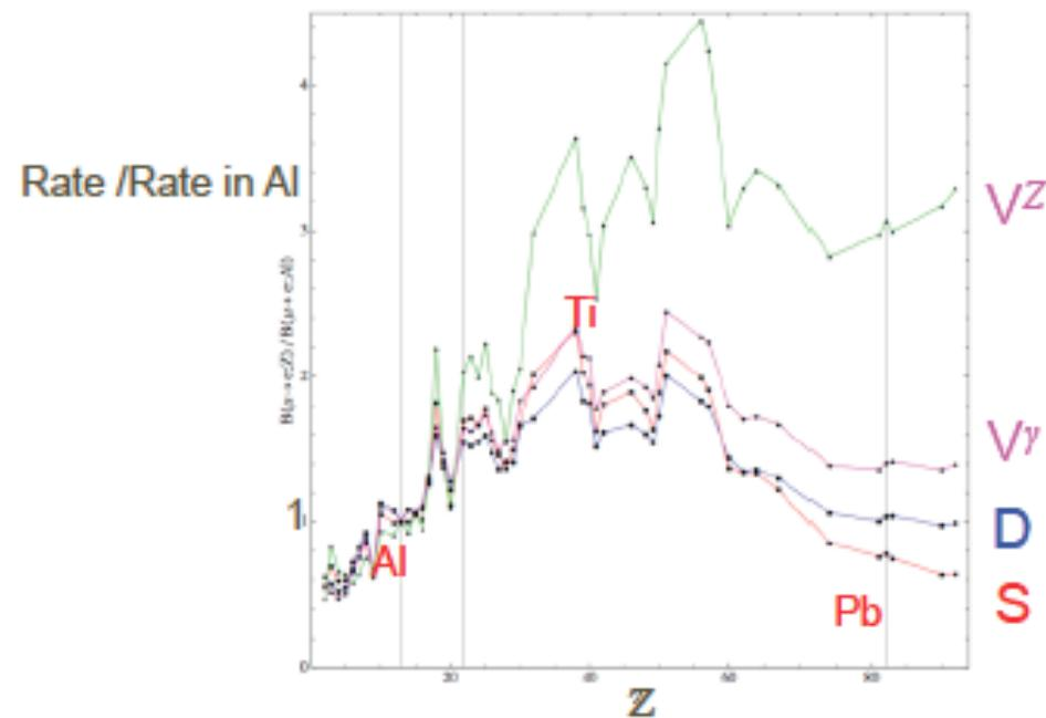
Figure 3: Target dependence of the  $\mu \rightarrow e$  conversion rate in different single-operator dominance models. We plot the conversion rates normalized to the rate in Aluminum ( $Z = 13$ ) versus the atomic number  $Z$  for the four theoretical models described in the text:  $D$  (blue),  $S$  (red),  $V^{(\gamma)}$  (magenta),  $V^{(Z)}$  (green). The vertical lines correspond to  $Z = 13$  (Al),  $Z = 22$  (Ti), and  $Z = 83$  (Pb).
