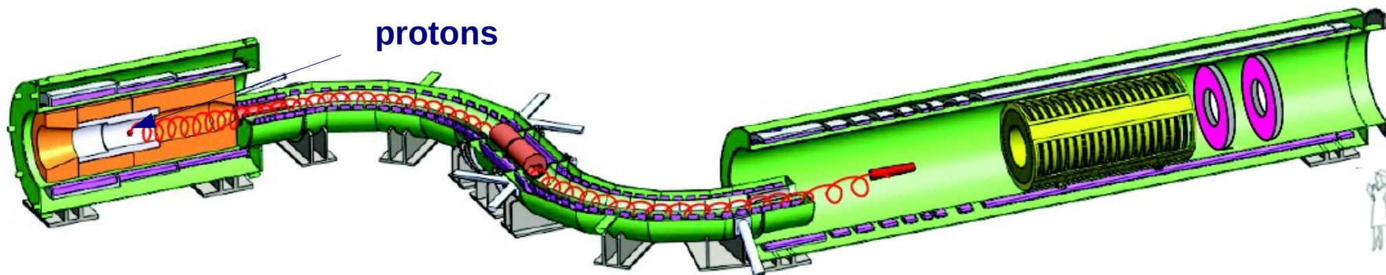
**Production Solenoid:** 8 GeV  $p$  on tungsten, graded field channels  $\pi$ ,  $K$  and  $\mu$  from their decays
