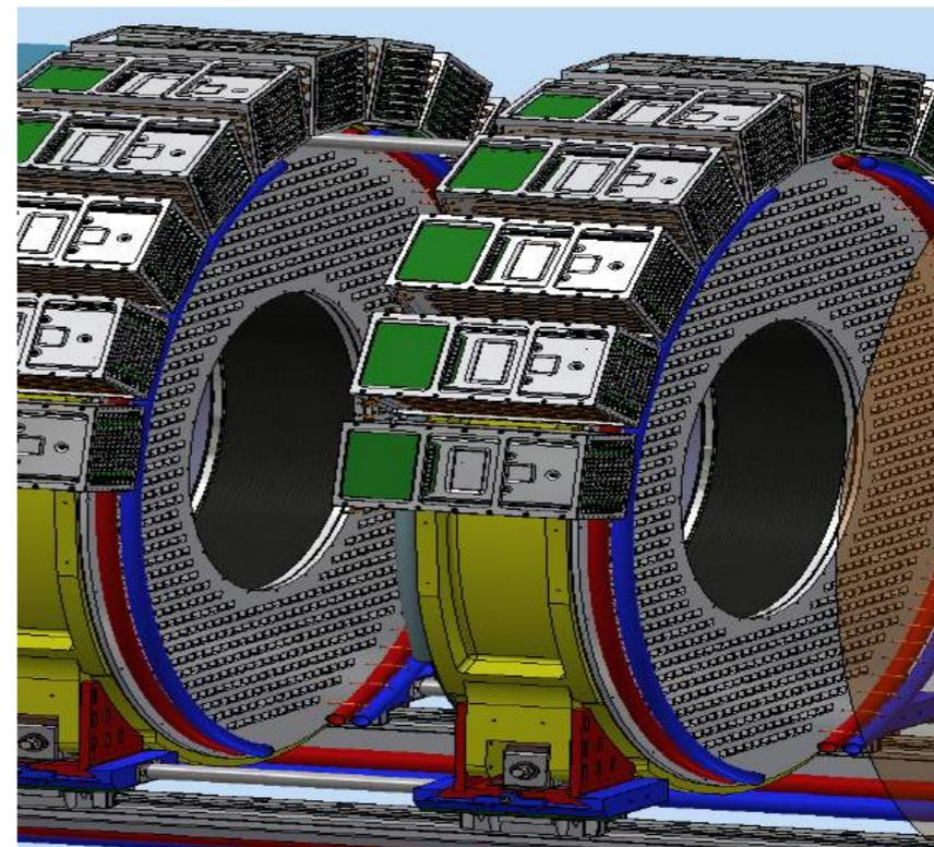
Each calorimeter disk consists of 674 CsI 34x34x200 mm<sup>3</sup> crystals
