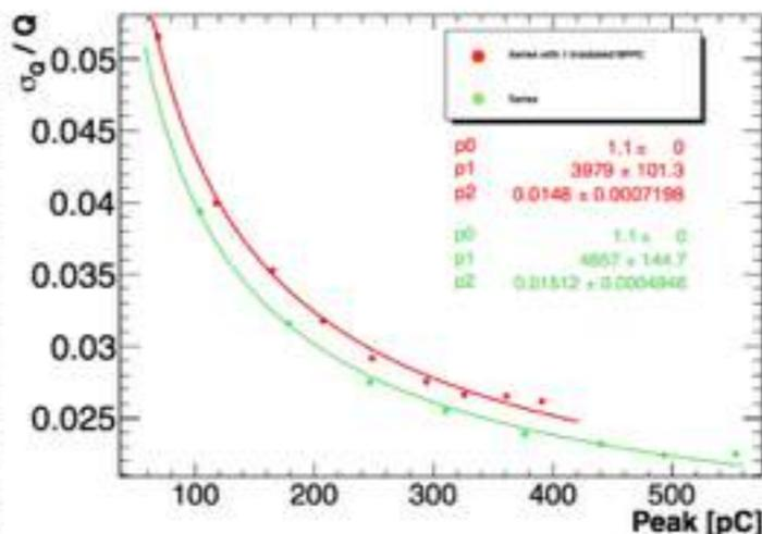
Resolution vs peak fitted with:  $\sqrt{F/(Q/A)}$
