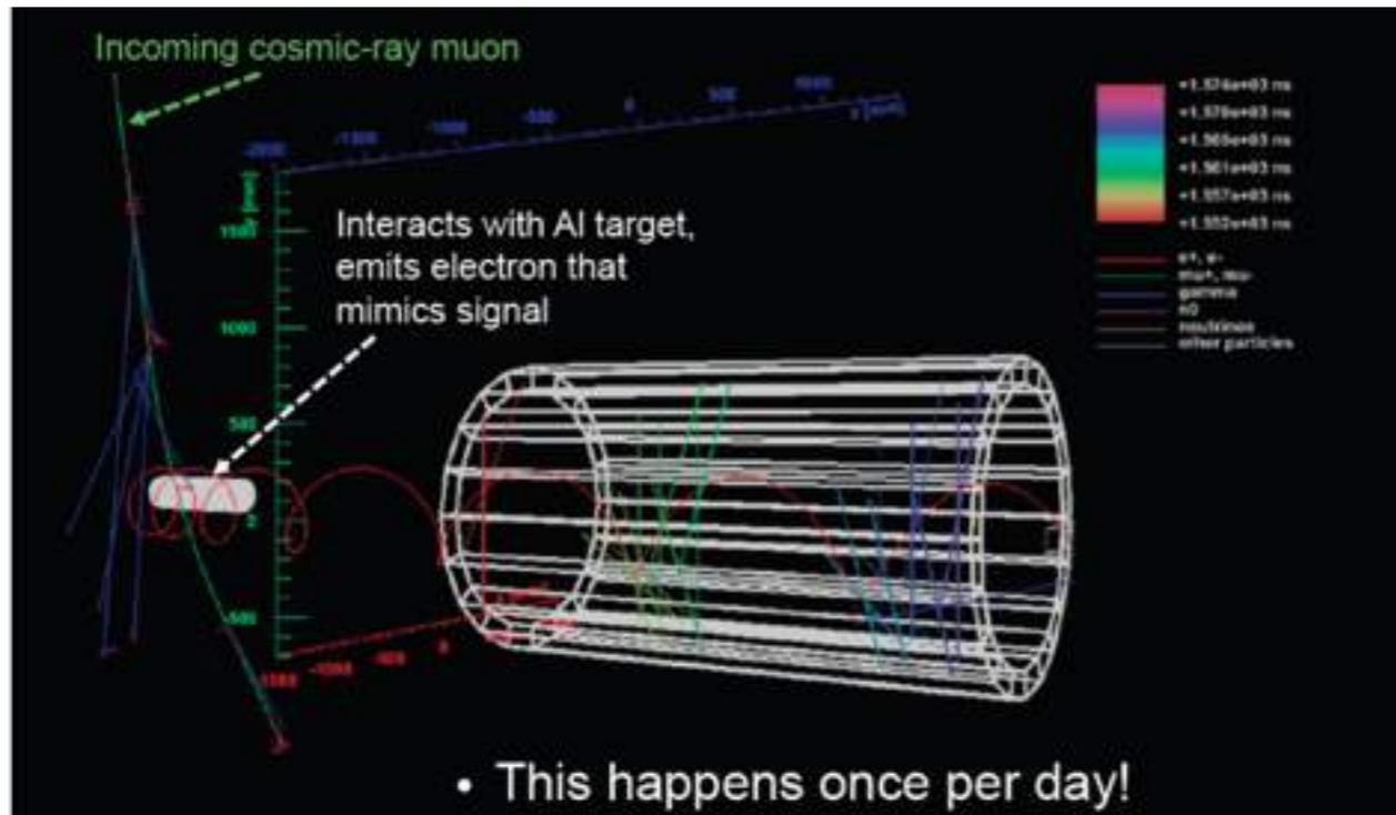
2.2 events with cosmic muons with  $103.5 < P < 105 \text{ MeV}/c$  enter the detector bypassing the CRV counters and surviving all analysis cuts.
