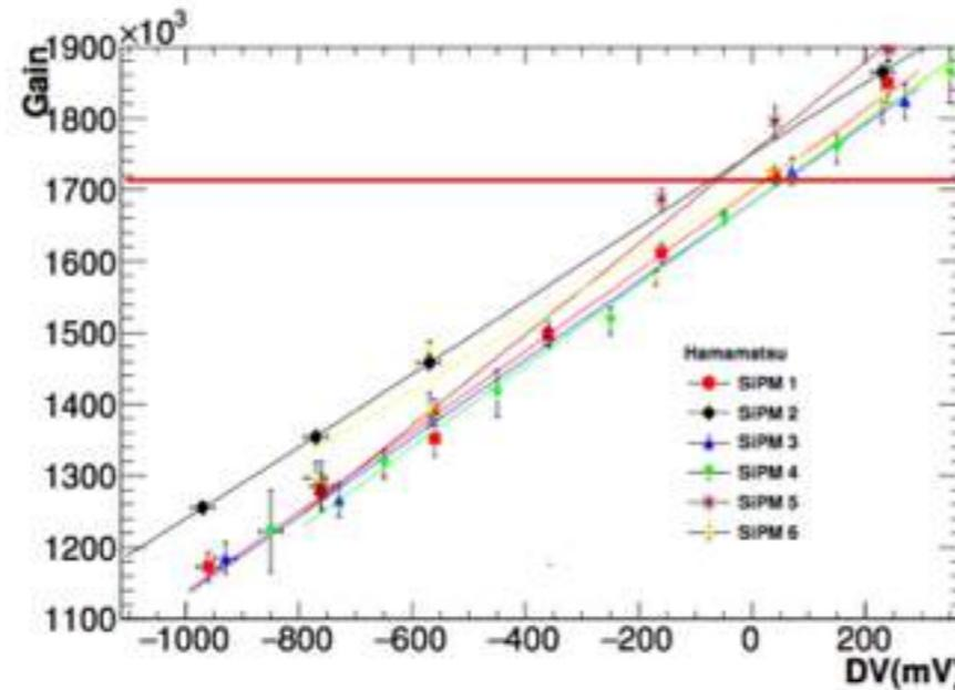
$$Q_n = G_{amp} \times G_{SiPM} \times N_{pe} \times e \Rightarrow G_{SiPM} = \frac{\Delta Q}{G_{amp} \times e}$$
