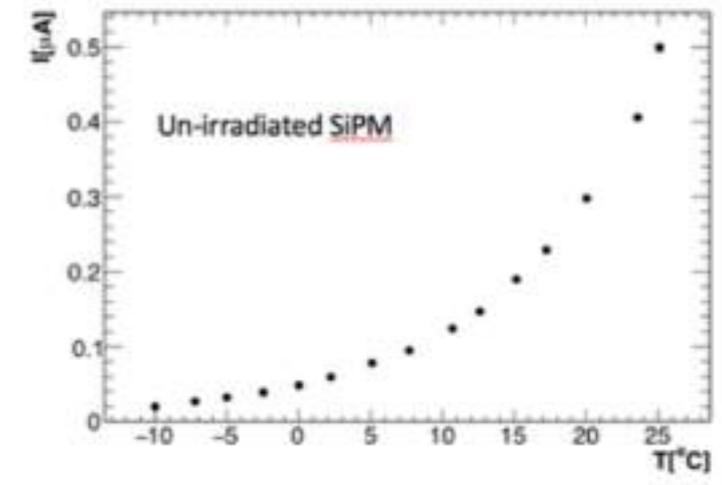
It is necessary to cool down the SiPM system at 0°C
