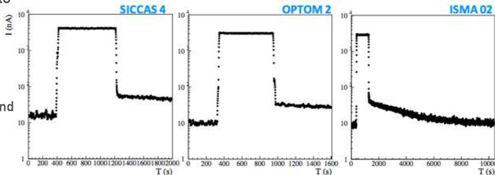
RIN from thermal neutrons in the hottest region: 60-85 keV. Well inside the Mu2e requirements (RIN < 0.6 MeV) ✓✓
