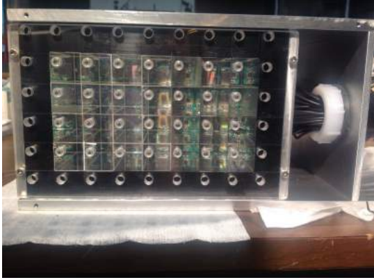
Figure 1: A prototype of the (g-2) -calorimeter, tested at SLAC. This test-box consisted of a 4 \times 7 \text{PbF}_2 crystal array with each crystal coupled to a Hamamatsu SiPM.
