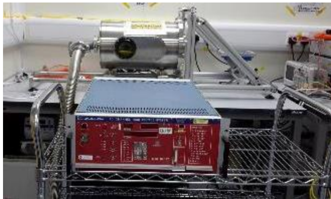
Vacuum Tank + HV for Module Testing In Liverpool prior to shipping to FNAL.
