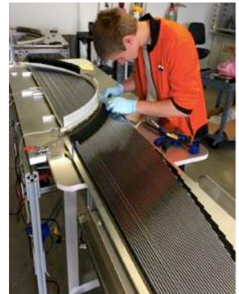
Panel: Straw Installation
