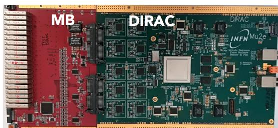
Figure 6: Picture of the electronic board used to manage and read out 20 SiPM+FEE channels.
