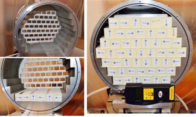
Figure 1: Pictures of Module-0 front view during assembly : mechanical structure (top left), crystals assembly (bottom left) and final version (right).
