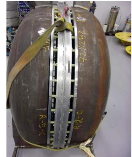
Cryostated Model Coil
