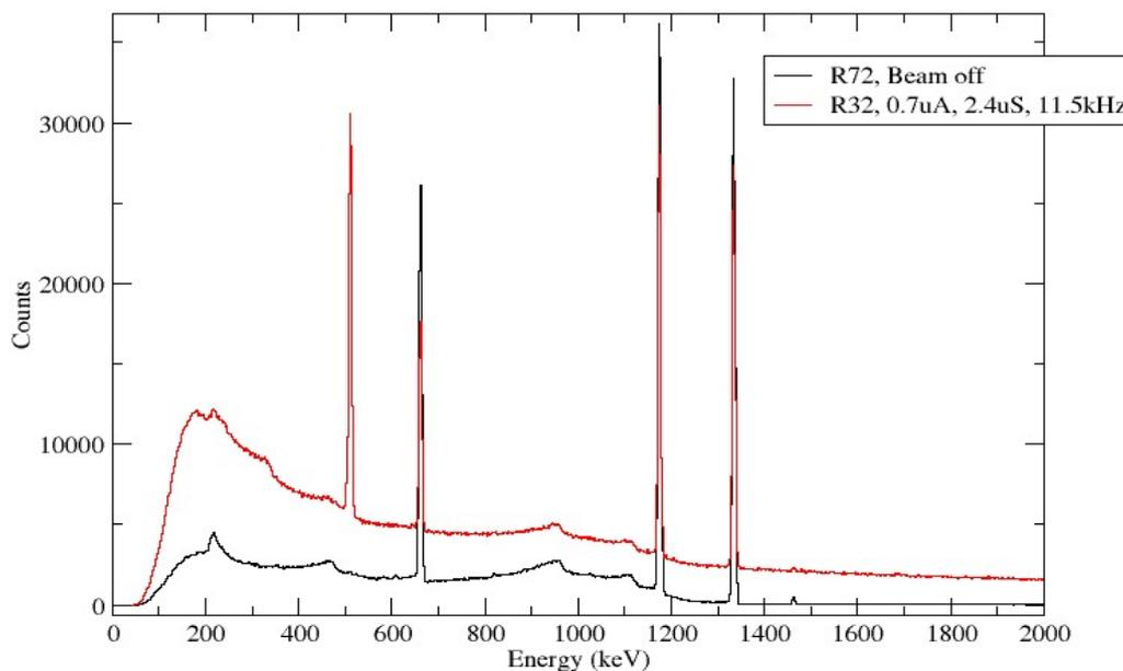
Figure 2: Example beam on and beam off energy spectra of photons produced in the experiment.
