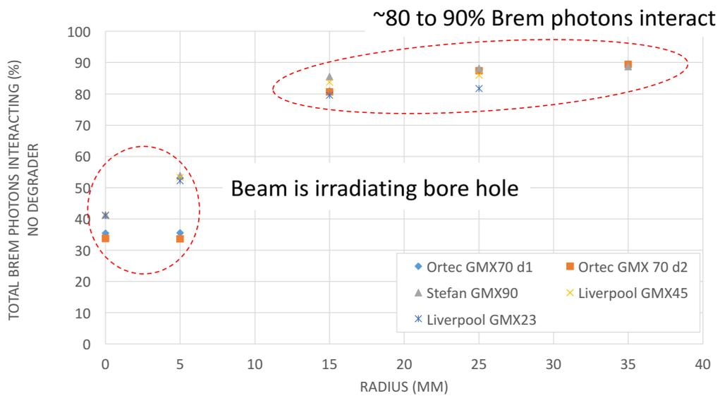
Figure 11 Total Brem photons interacting as a function of radius, for various GMX detectors, no degrader
