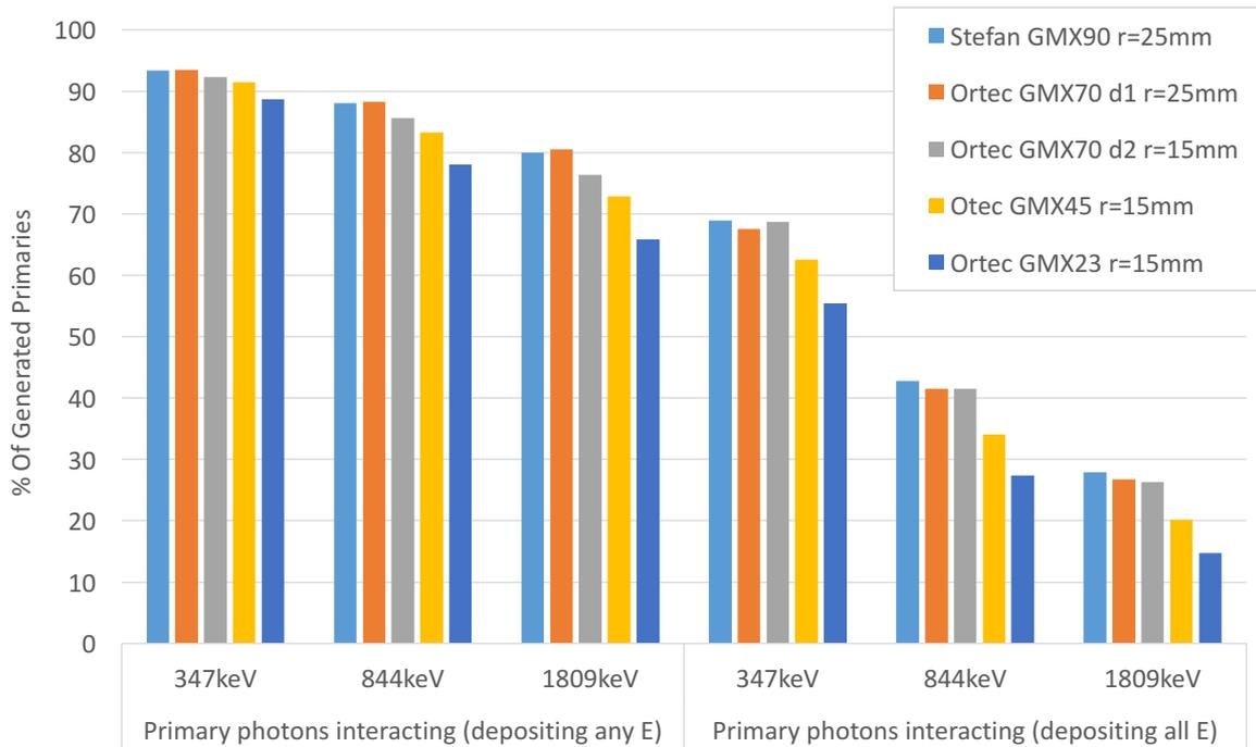
Figure 14 Detector efficiencies for the various detectors and 3 photon energies of interest. Only those photons that deposit all E will be used in analysis.
