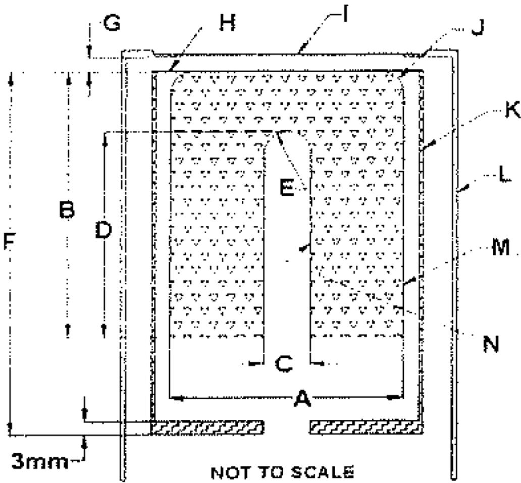
Figure 9 General drawing of a HPGe detector (Ortec Website)
