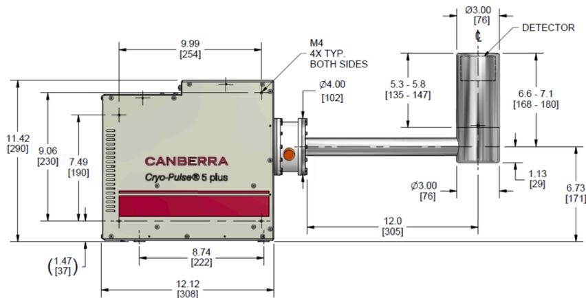
**CP5-PLUS-U Electrically-Cooled Cryostat (side view)**
