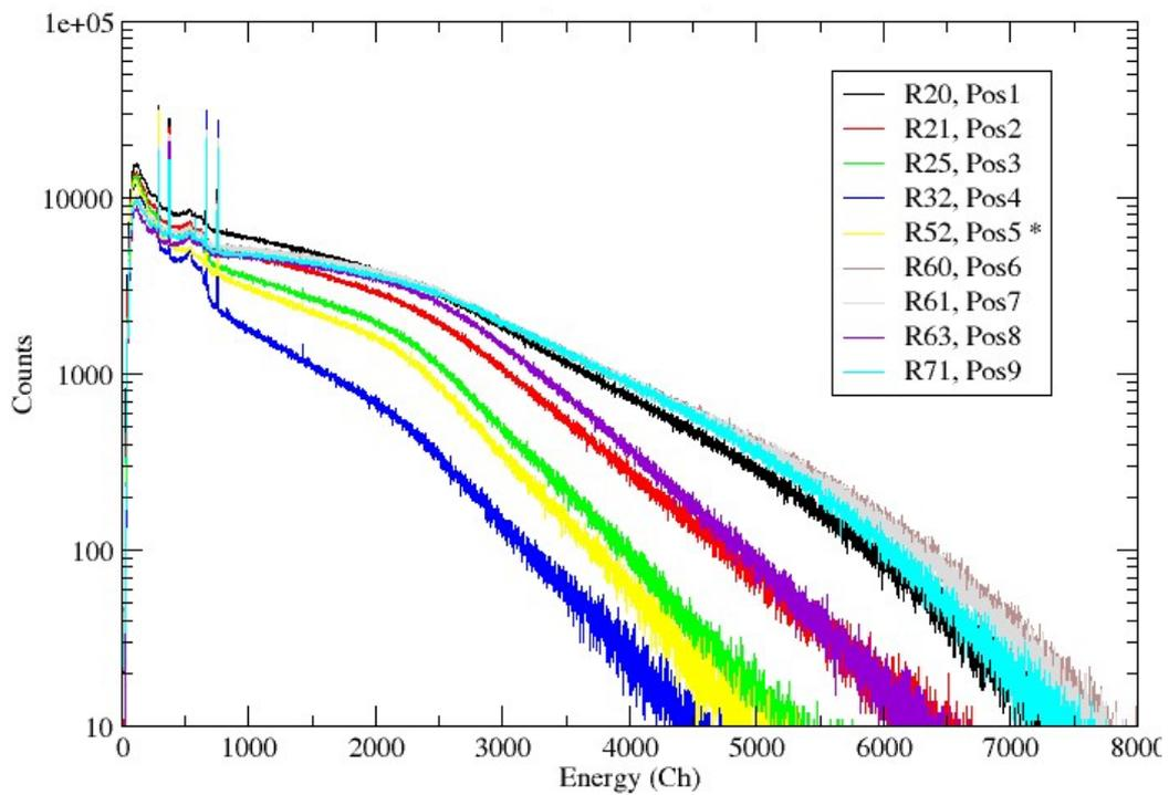
Figure 5 Energy spectra for a fixed beam rate but with the detector in different orientations
