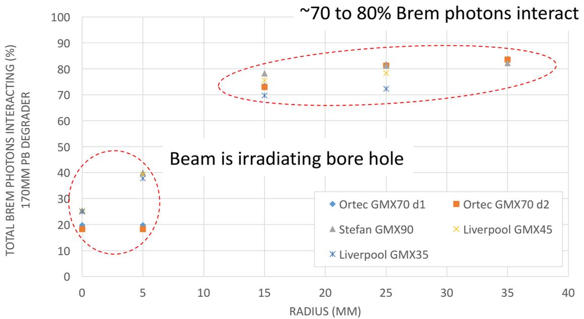
Figure 13 Total brems photons interacting as a function of radius for various GMX detectors, 170mm Poly degrader
