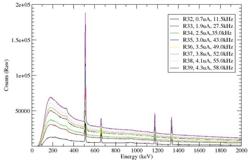
Figure 3 Example energy spectra for various beam rates
