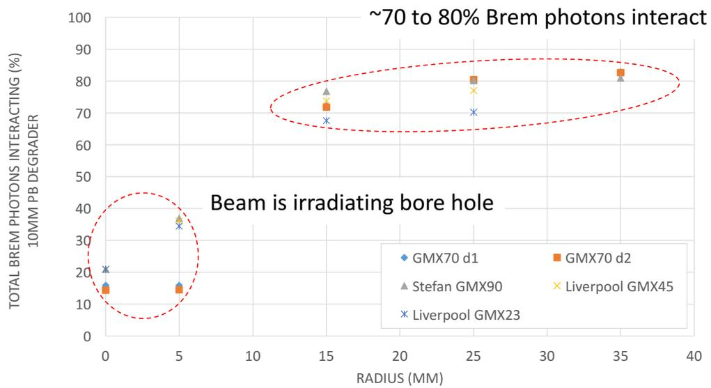
Figure 12 Total Brem photons interacting as a function of radius, for various GMX detectors, 10mm Pb degrader
