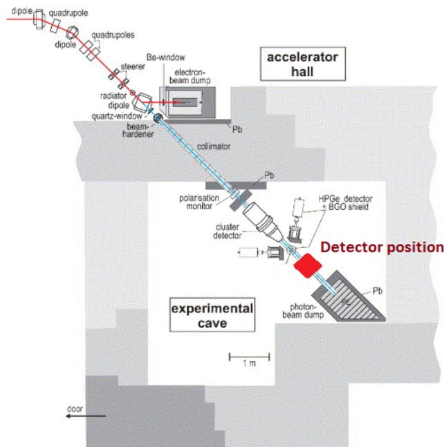
Figure 1: Detector Position in ELBE Experimental Cave
