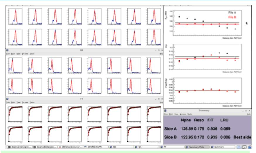
Example of "QA-USER" page for source scan of a single crystal on both readout sides
