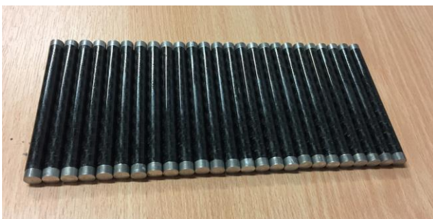
Figure 17: Carbon fibre posts, one of which was added to each module.
