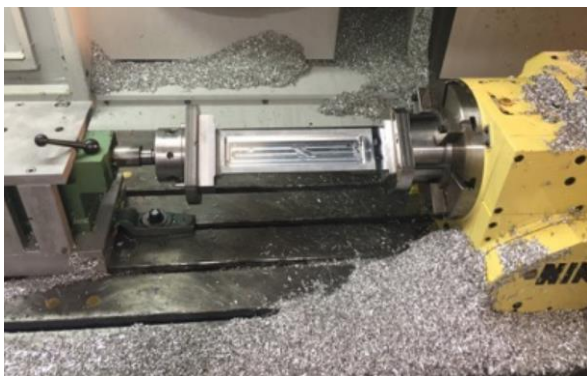
Figure 6: Production of tracker module manifolds, lids and snouts in the Liverpool workshop.
