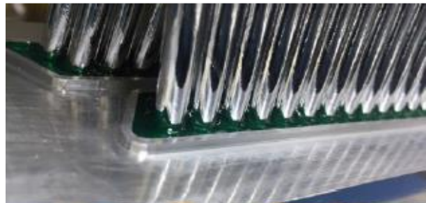
Figure 12: Straw ends glued into manifolds.
