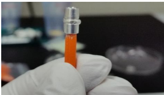
Figure 13: Gluing of aluminium endpiece.
