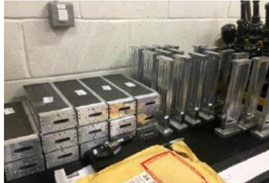
Figure 6: Production of tracker module manifolds, lids and snouts in the Liverpool workshop.
