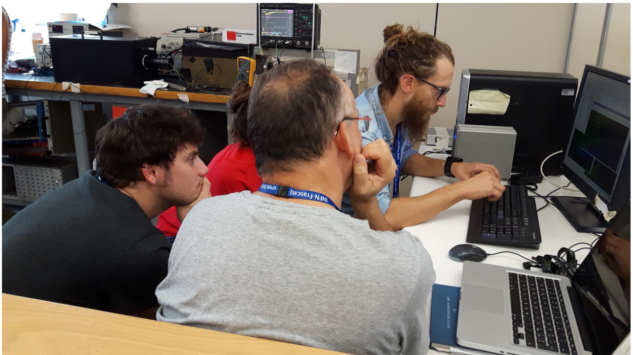
Figure 3: Test of scintillating crystals during the 2017 edition of Incontri di Fisica. On the left, the black tight-box used to test crystals is visible. Participants are analysing data to evaluate the optical properties of CsI crystals.
