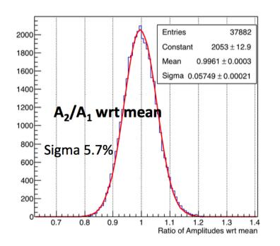
Distribution light stability measured as ratio of the LM's pulse amplitude
