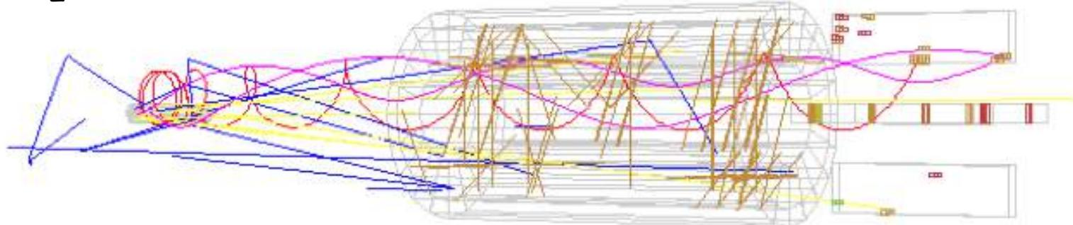
Search for tracking hits with time and azimuthal angle compatible with the calo clusters ( $|\Delta t| < 50$  ns) → **simpler pattern recognition + higher efficiency**
