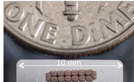
Cross-section of Extruded TS Conductor
