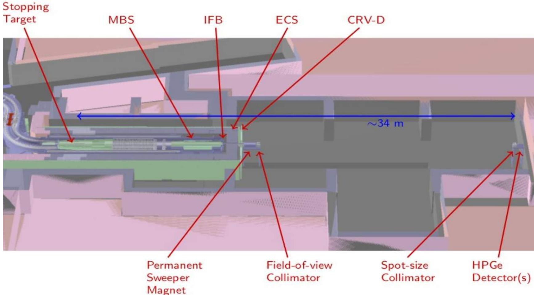
The STM will measure a variety of well understood gamma ray lines ... under a high-rate brehmstrahlung background
