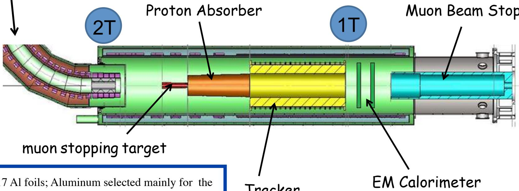
17 Al foils; Aluminum selected mainly for the muon lifetime in capture events (**864 ns**) that matches nicely the prompt separation in the Mu2e beam structure.
