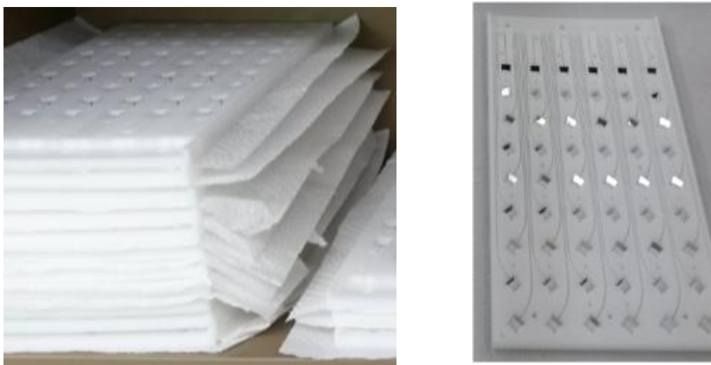
Figure 6. Light distribution plates before and after gluing of right-angle prism.
