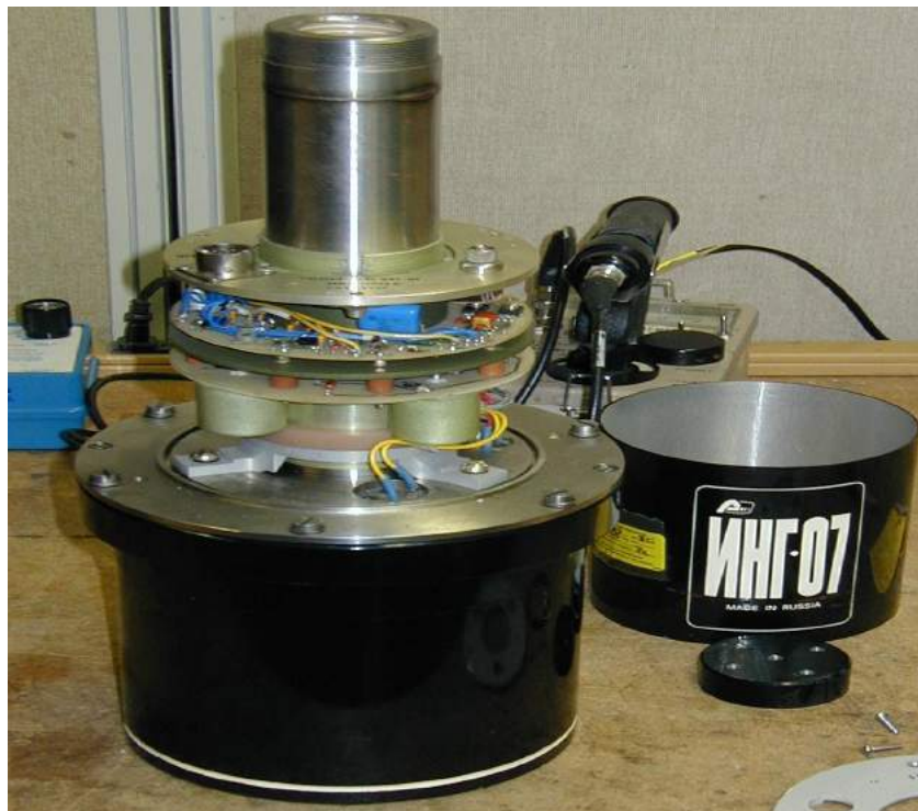
Figure 7.8 The model ING-07 DT generator salvaged from BaBar and in use in the Mu2e prototype source calibration system.
