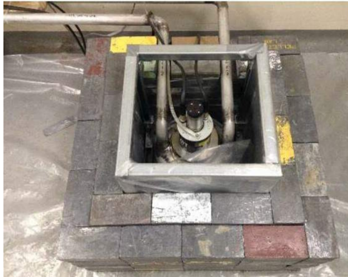
Figure 7.10. The DT generator in place in the Fluorinert bath in the partially constructed prototype source bunker.
