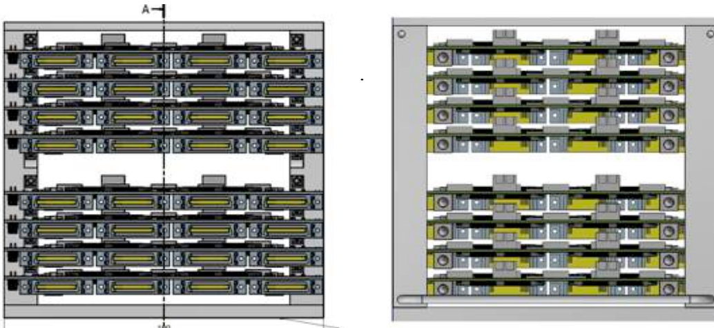
Figure 6.25: (Left) Rear, (right) front view of a readout crate with MB/WD boards mounted.
