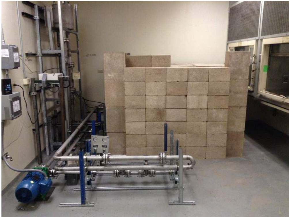
Figure 7.9. The prototype source calibration system at Caltech. The DT generator and Fluorinert bath are hidden in the bunker. The refurbished circulation pump is in the lower left with its associated controls and power source above. The reservoir is visible in the upper left of the picture. The “test” section, where crystals may be irradiated, is the section of plumbing between the two flanges in the front.
