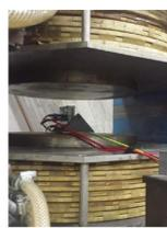
The DCDC behaviour in magnetic field was tested for different orientations at the LASA INFN laboratory of Milan Italy.
