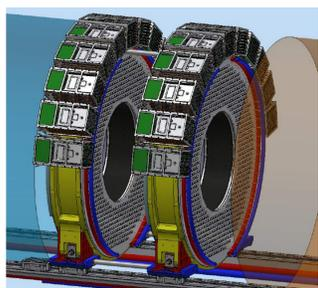
Each crystal is coupled to two  $14 \times 20 \text{ mm}^2$  large area UV-extended SiPM, for a total of 2694 electronics channels. Photosensors are packed using a parallel arrangement of two groups of three cells biased in series.
