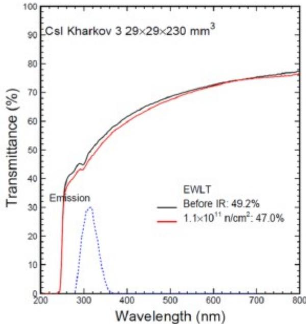
← Emission Weighted Longitudinal Transmittance (EWLT) ~50%
