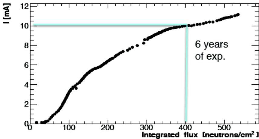
← Dark current after n radiation (no damage from dose)
